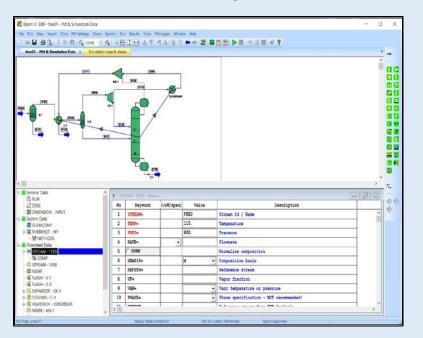
This interface provides a seamless bridge between the historical keyword input language of process simulators and the graphic windows interface which enables the drawing of process flow diagrams with unit-operation symbols and connecting streams. Graphics functions allow the user to manage a large number of graphical results especially when dynamic simulation studies are developed.
